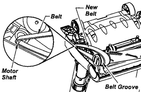
**NOTE:** Care must be taken due to the belt tension during reassembly.
